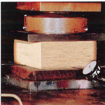
EXAMPLES OF WJE COMPRESSION TESTS ON VOSS ENGINEERING EXPANSION BEARING PADS
